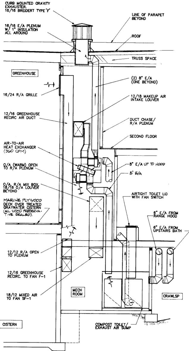
VENT SYSTEM – SECTION THROUGH CHASE
